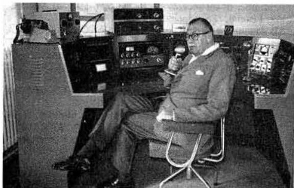
The station of Arland Ussher, GD3TIU, at Crosby, Isle of Man. The equipment includes an HT41, HT32 and a 75A4. The aerial system consists of five Vee beams each leg being 344 ft long. Arland also holds the call ZS6Z and was the President of the South African Radio League between 1938 and 1950.
